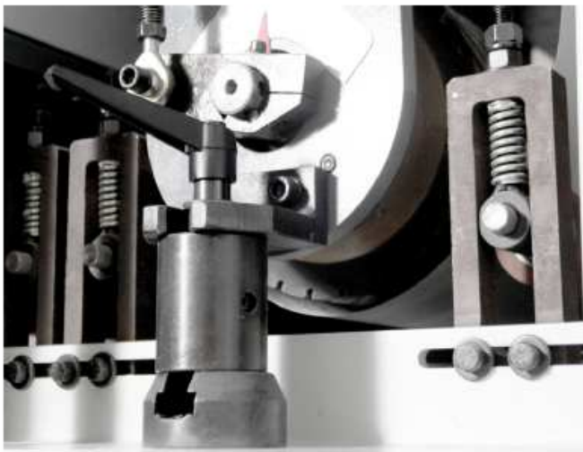
Quick lock for easy changing of sanding paper
