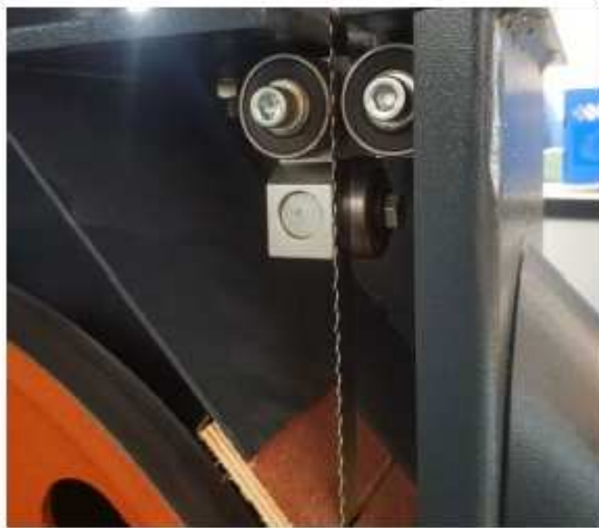
All European model blade guiding system for high precision running
