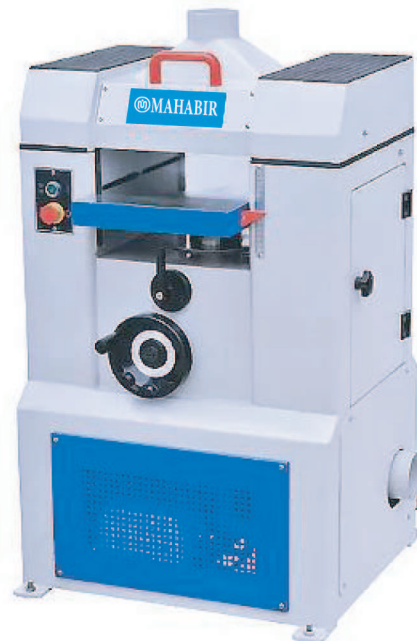
MBZ1010/1013 is automatic setting model professional heavy model, planing width reaches 1000mm to 1300mm
