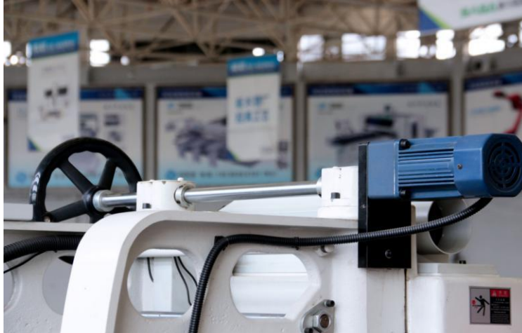
Automatic thickness adjusting
