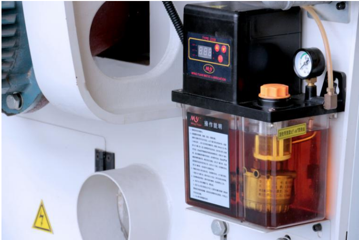
Automatic lubrication system to make sure all mechanical movement is smooth, and it spread oil to main spindle to make sure the spindle is lifelong use
