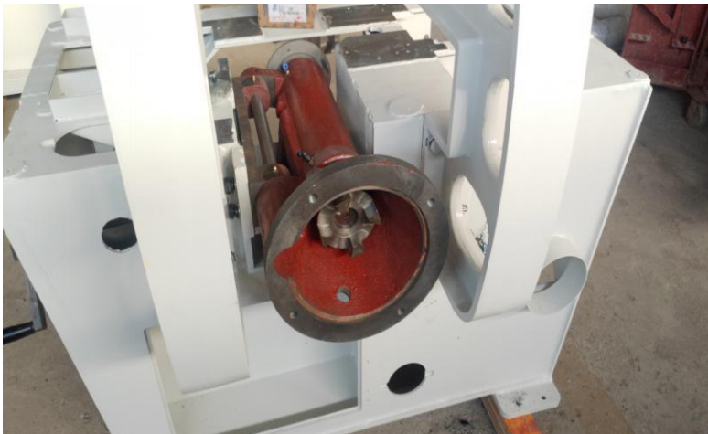
Heavy duty cast iron spindle
