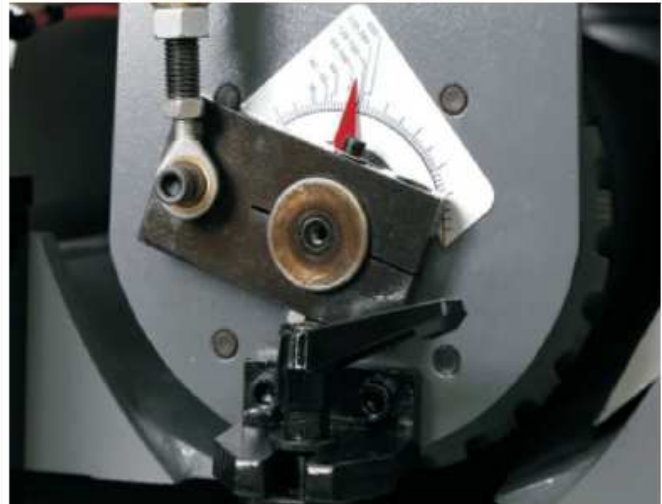
Each sanding shaft got separate sanding scale setting function
