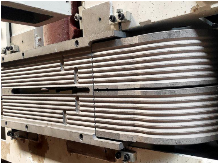
Low temperature nitriding treated feeding rail, unti years friction without change precision
