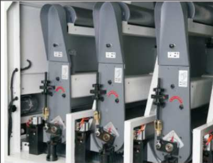
3 sanding shaft for flexible grit sanding
